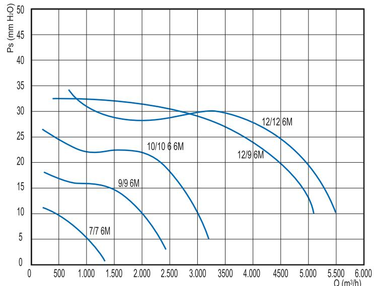
6 poli/poles (1000 rpm) T: trifase/three-phase (400V-50 Hz)
