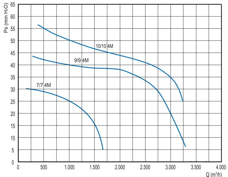
6 poli/poles (1000 rpm) M: monofase / single-phase (230V-50 Hz)
